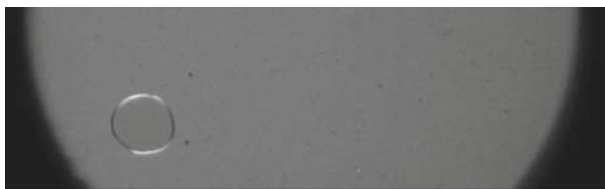
Fig. 8 Photo through a microscope after a pulse having a fluence of about 1,000 \text{ J} \cdot \text{m}^{-2} . The cavitation regime takes place at this fluence value. The maximum bubble diameter is 140 \mu\text{m}
